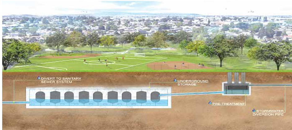
RENDITION of the Multi-Benefit Stormwater Capture Project which consists of a 6.4-million-gallon capture system almost entirely underneath the park.
